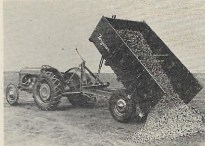
MANURE SPREADER and TRAILER — Both use exclusive Ferguson trailer hitch which increases traction by distributing a portion of the load to all four wheels of the tractor.
