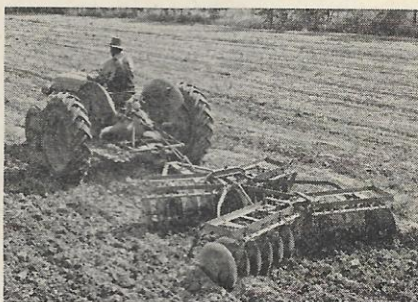
DISC HARROWS — Tandem or single — angle of discs hydraulically controlled.
