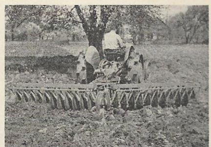
DISC HARROWS — Tandem or single — angle of discs hydraulically controlled.
